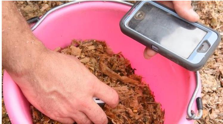
The preferred method for a SCiO device is to collect a forage sample in a pail. Using the ground or face of the pile directly can alter your scan results.
