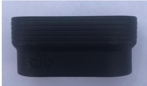
Once connected, using the optical shade is imperative for success while scanning. The device is ultimately reading a light beam that passes through the forage. Scanning inside the pail and using the optical shade both help to keep outside light from interfering with your sample results.
